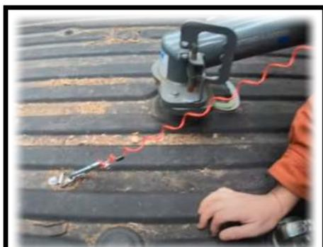
*The most important thing about a trailer breakaway system is that the cable be attached to the towing vehicle*
